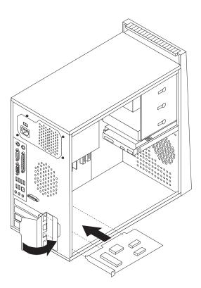
Figure 9. Closing the PCI card latch
